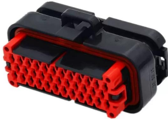
Controller Interface Definitions (35Pin, AMP776164-1)
